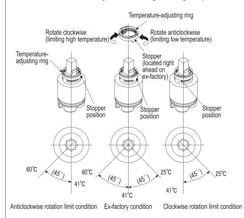
⚠ Attentions: The temperature is a reference value. The water entry temperature reference value is Tc = 25 oC, Th = 60 oC.
