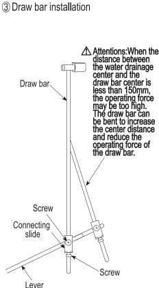
a.As shown in the diagram, first put the lever through the connecting slide. Then use connecting nut to secure the draw bar and connecting bar. Adjust the position of the connecting slide to make the lever and water stop plug be in an appropriate position and secure with screw.
