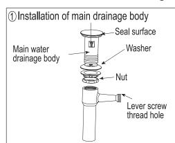
a.Remove the water drainage head and seal ring from the main water drainage body.
