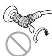
Do not open or close the shutoff valve when setting. /
