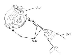
后背吊钩的安装方法/ Back hanger installation method
