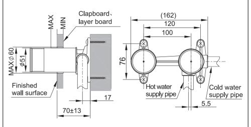
As shown in the figure, use screws to fix the product on the wall. \*\*Please according to the need to further prepare suitable screw.
