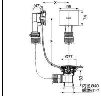
DB602N-1A 400 < x+y < 485 DB602N-2A 485 < x+y < 585 DB602N-3A 585 < x+y < 685
