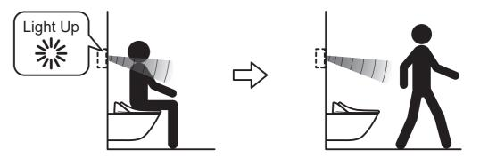
If an obstacle is sensed for more than 10 minutes, wait for the distance automatically adjusted.
