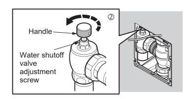
Depending on installation conditions, such as on-site water pressure, a pulsating sound may be generated because of the characteristics of the constant flow valve; this is not abnormal. If the noise is bothersome, the noise may reduced by turning the water shutoff valve off.
