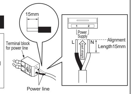
Make the core wires of the power cable the same length (the length of the exposed power terminal block should also be the same).  Insert the wire core straight into the power terminal block.
