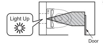
\*If the sensor detects a wall or door, it will not be able to accurately detect the human body and will not be able to determine large or small washing or perform automatic washing.
