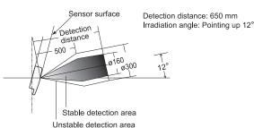
Irradiation angle and detection area \* For a 300 x 300 mm blank white paper
