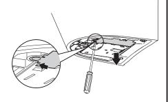
控制器无法降下时,请使用平头螺丝刀将其拆下/ If the controller does not slide out on its own, use a flat-head screwdriver to lower it.
