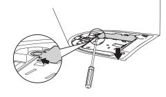
控制器无法降下时,请使用平头螺丝刀将其拆下/ If the controller does not slide out on its own, use a flat-head screwdriver to lower it.
