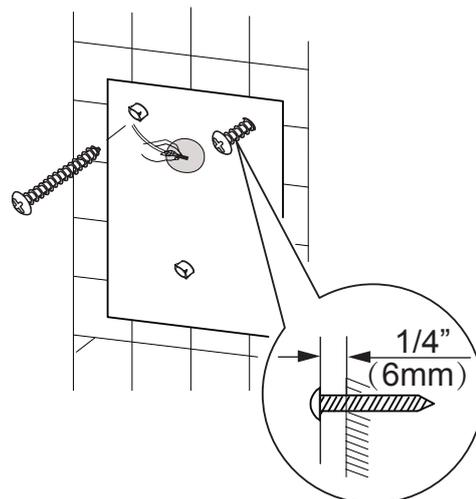
4.Insert self-tapping screws into the upper
