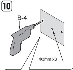
When mounting on a plaster board or tiled wall.
